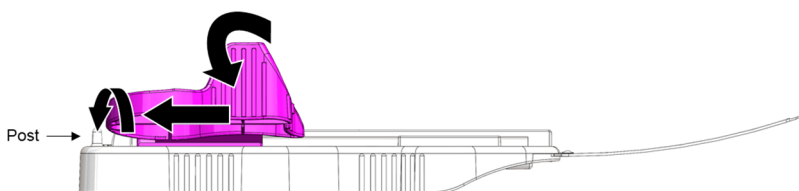
Figure 8: Rotate Blade Handle down and move proximally to the locked position on the Post
